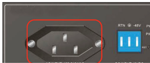
Figure 4-7. Inserting the AC power cord into the AC socket to power on this switch.
